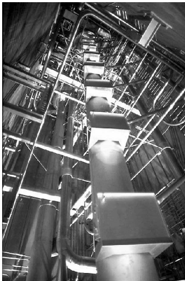
FIGURE 3 Pulsed column. The boxes around the column contain sensors that measure the progress of the extraction. Photograph courtesy of COGEMA.
