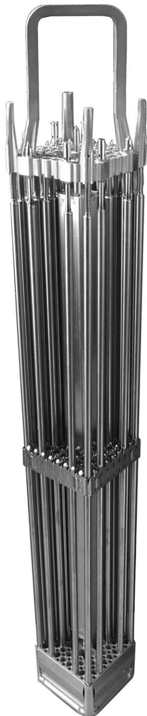
FIGURE 1 Boiling water reactor fuel assembly. Some fuel elements have been removed to show more structural detail. Photograph courtesy of Framatome.
