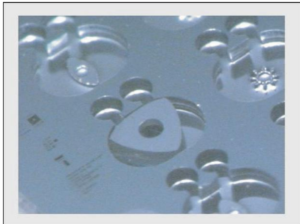
FIGURE 3 Lithographically deined 1-mm Wankel rotor in its housing. (Courtesy of University of California, Berkeley.)
